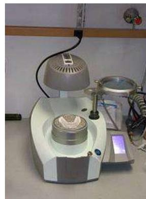
Figure 1: Erkoformer computerized "Sudden Vacuum" pre-charged pump chamber former from Glidewell Labs.
