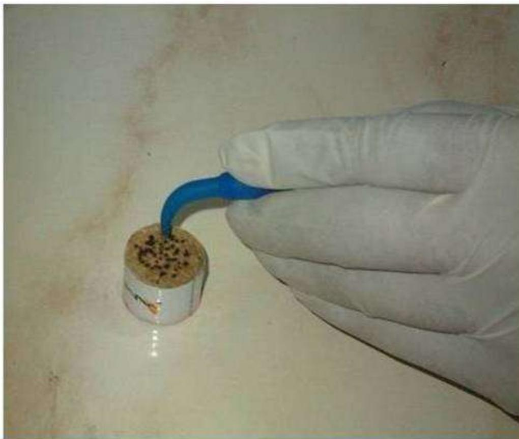
**FIGURE 2: Conditioning or priming of fibre tip on a wooden cork**
